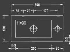
Thickwalled, low hand-washbasin in ceramic, without putdown space, inside depth 60 mm. Option of leftside taphole (.B).
