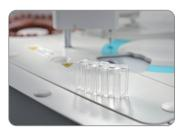
40 disposable cuvettes 100µl minimum reaction volume
