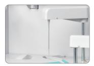
Liquid level detection, vertical collision protection for probes and inventory checking
