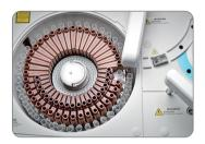
40 positions for reagents 40 positions for samples Built-in barcode reader
