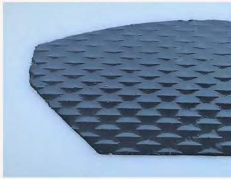
Structured surface from die-casting
