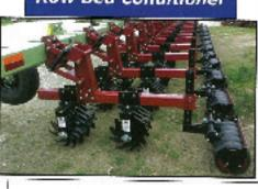
Heavy Duty Parallel Linkage is Designed Around Full Length Greasable Bushings Easily Adjustable Row Unit Down Force
