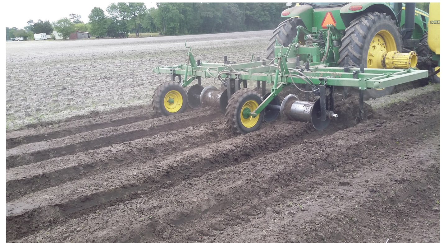
Britt Farms 4 Row 40" hydraulically powered cone roller
