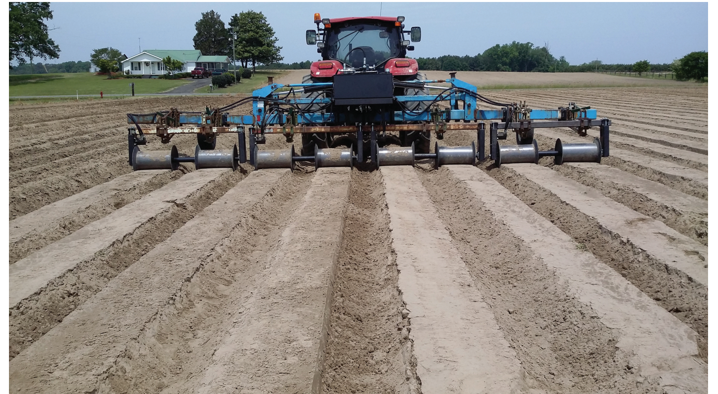
Above: 8 Row 22" wide rollers, 14" in diameter with 20" cone disc blades on 40" rows
