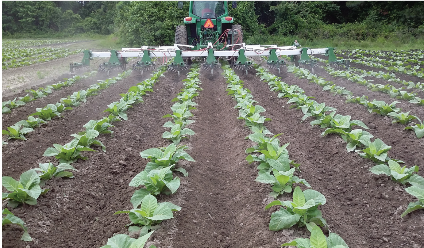
Top: Millstream Farm's 8 Row 44" PATS Cultivator on KMC Stacking Toolbar.
