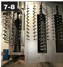
**7-8** A 200 MPH air blast removes water drops from the pre-treated aluminum. A convection oven completes the dry-off process.
