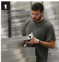
**1** The raw premium-grade aluminum is inspected to be free of blemishes and is not exposed to the outdoor elements.
