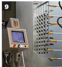
**9** Powder is applied with 18 automated and 2 manual spray guns. Compressed process air is dried to -35°F Dew Point for superior adhesion.
