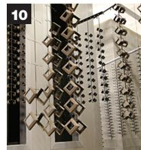
**10** The powder coating is then bonded and adhered to the aluminum substrate in a 400 degree cure stage.
