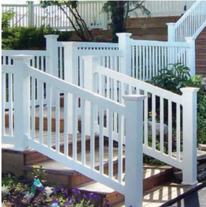
Standard Baluster 7/8" x 1-1/2" Rectangular Vinyl 2-7/8" Baluster Spacing
