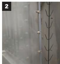
**2** The product enters a heated acidic cleaning stage to remove extrusion debris and fabrication oils.
