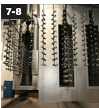
**7-8** A 200 MPH air blast removes water drops from the pre-treated aluminum. A convection oven completes the dry-off process.
