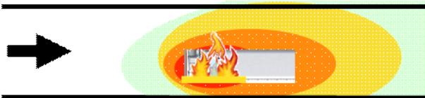
Fig. 6: Schematic view of area with high temperatures during a truck fire with FFFS
