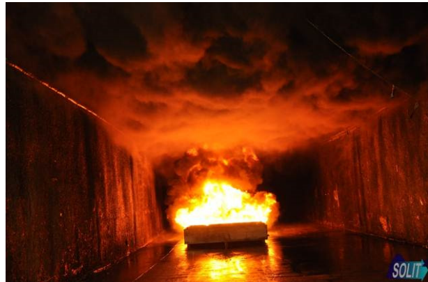
Fig. 20: Layer of smoke in a 30 MW liquid fire shortly after ignition.
