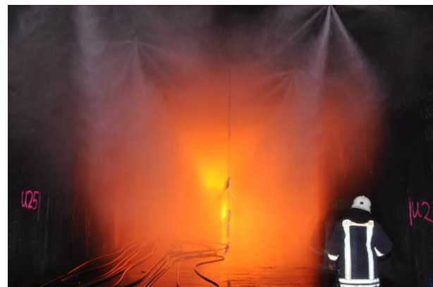
Fig.30: Typical view of a fire fighter looking at the source of the fire (approx. 40 MW) from a distance of 20 m with an activated water mist extinguishing system
