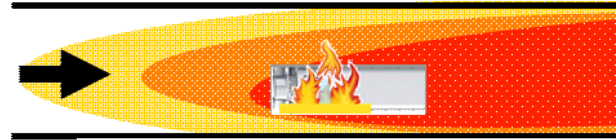
Fig. 7: Schematic view of area with high temperatures during a truck fire without FFFS
