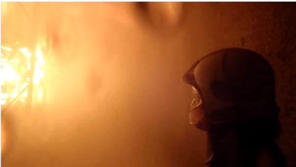
Fig. 27: Firefighter in the direct proximity of a truck fire with activated water mist system
