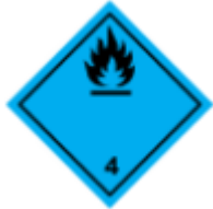
Figure 4: Pictogram of Dangerous Goods Class 4.3 for substances, which form flammable gases in contact with water
