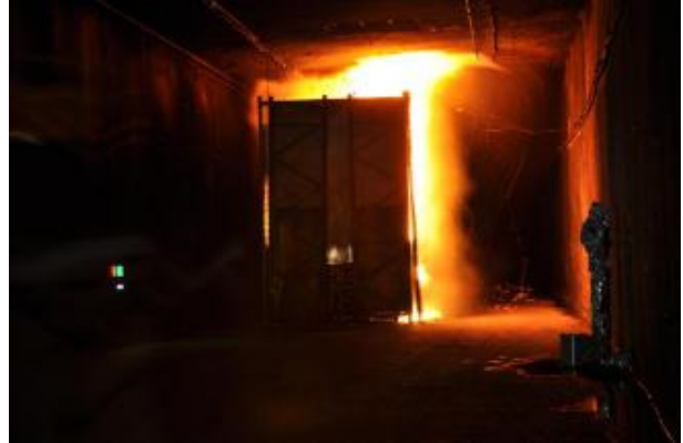
Figure 8: SOLIT Truck Fire Load shortly before activating the FFBS
