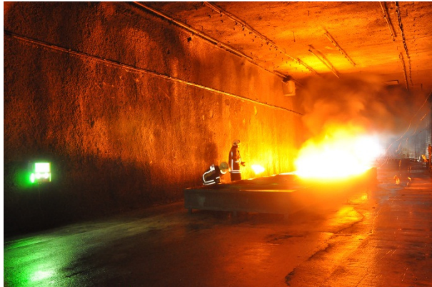
Figure 25: Ignition of the 60 MW pool
