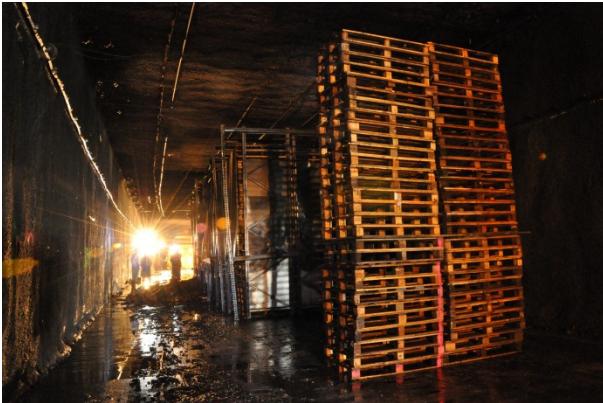
Figure 16: Target object after a fire test with a SOLIT truck fire load
