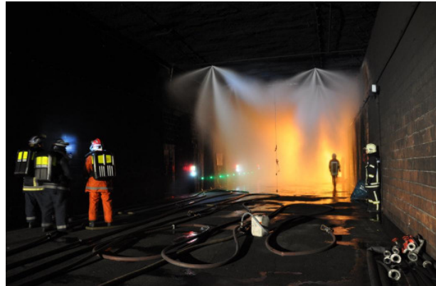
Figure 17: Upstream side of a SOLIT Class A fire load during the fire test.
