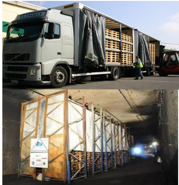
Figure 2. Euro pallets in transportation and as fire load in tests
