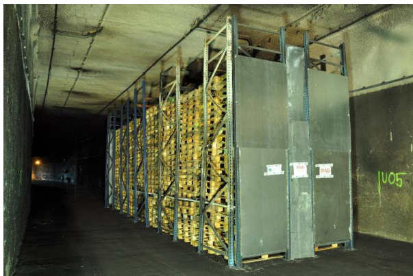
Figure 7. HGV mock-up without tarpaulin [18]
