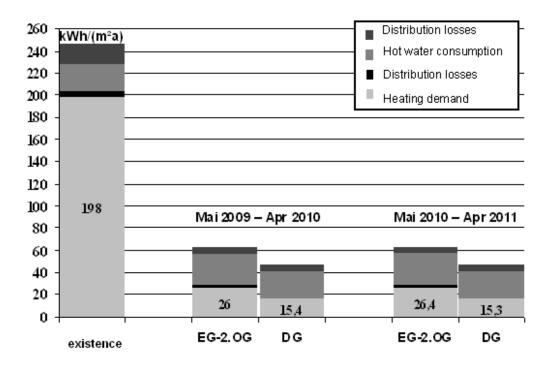
Figure 3: Final energy consumption (heating and hot water) for the renovated parts of the building (EG-2. OG) and the new Passive House attic apartments (DG).
