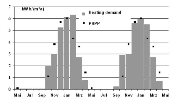
Figure 2: Heating demand for the renovated parts of the building, ground floor to second floor, for the first two time periods from May 2009 to April 2011; the 26 kWh/(m<sup>2</sup>a) calculated with PHPP was achieved despite two harsh winters.
