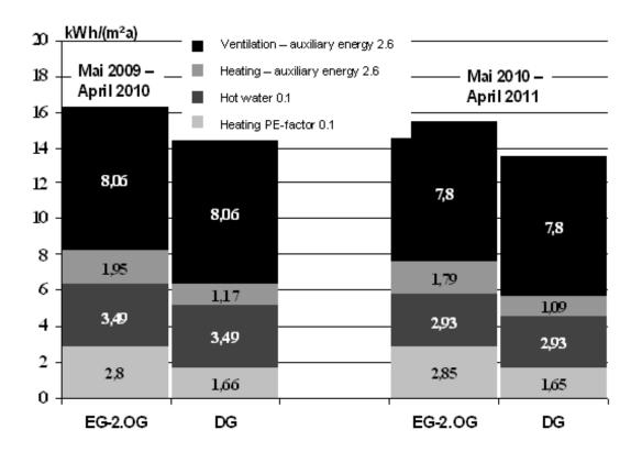
Figure 4: Primary energy consumption for renovated areas (EG-2.OG) and Passive House attic apartments (DG).
