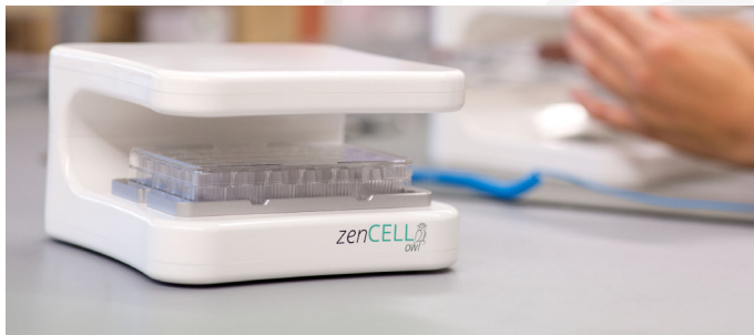
Figure 1: zenCELL owl, 24-channel microscope with 24-well cell culture plate.
