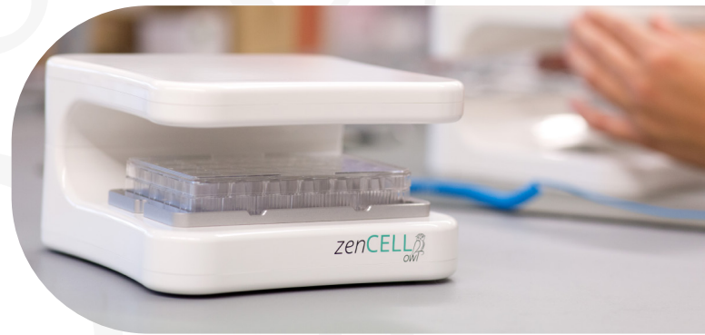
Figure 1: zenCELL owl. 24-channel microscope with 24-well cell culture plate.
