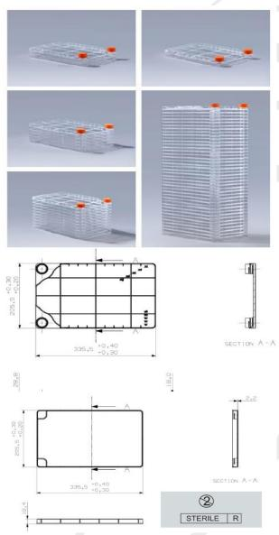
**Description:** Cell factory, one layer, two-layer, five-layer, ten-layer, forty-layer. TC treated (adherent culture) / Non-TC treated (suspension culture); Vent cap / seal cap, Sterilization (Gamma 25 kGy)
